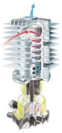
Condensate runs down to the bottom of the unit for automatic removal by the integrated drain valve.
