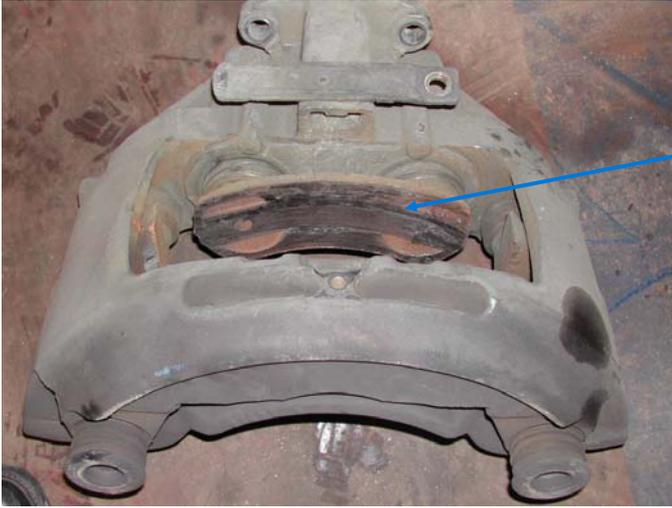
The thrust plate has been in contact with the disc = worn out pads, including the back plate! (Inspections?)
